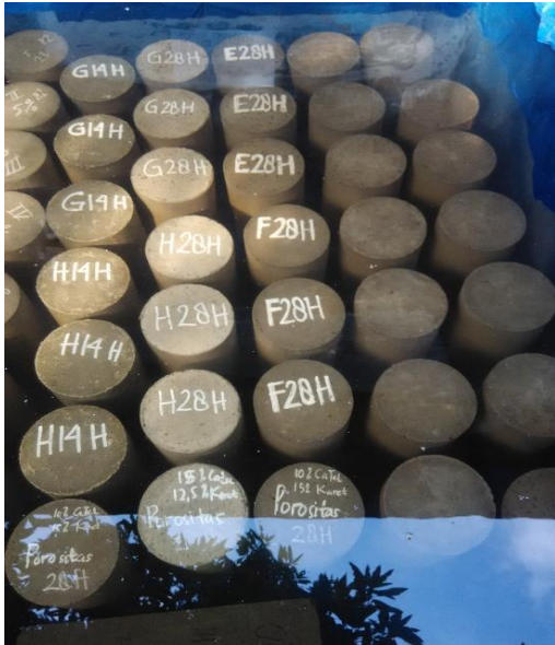
Perawatan Beton ( Curing )
