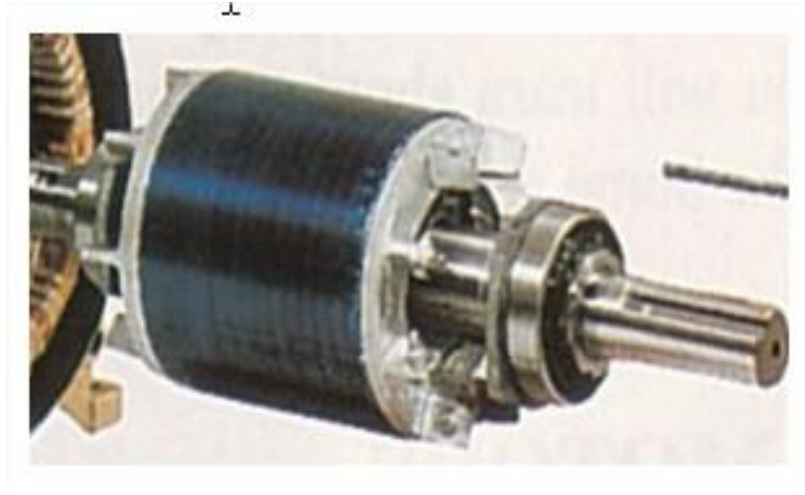
Gambar 2.5 Rotor Sangkar Tupai
