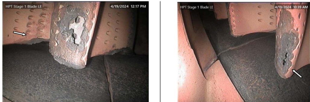
Gambar 4.4 Kerusakan HPT Stage 1 MPP Lombok
