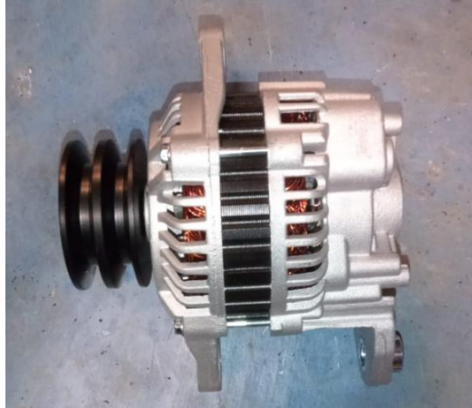
Gambar 2.3 Alternator Mesin Mitsubishi S16R PTA-S
