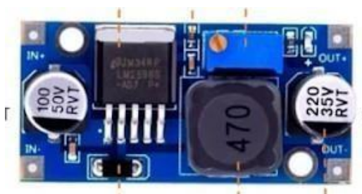
Gambar 2. 7 Modul Stepdown 12V – 5V LM2596. [24]
