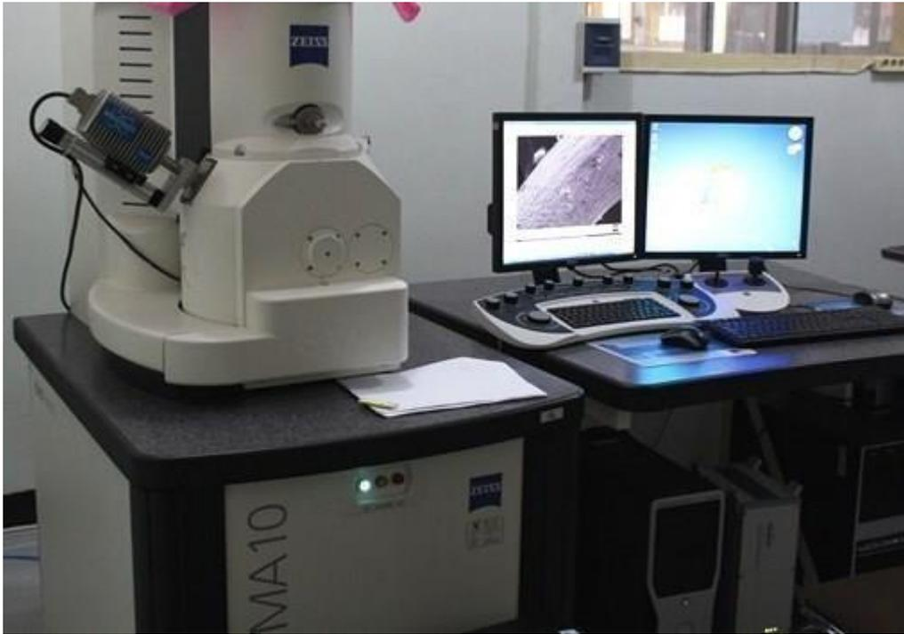
*Gambar 2.14 Alat scanning (SEM)*
