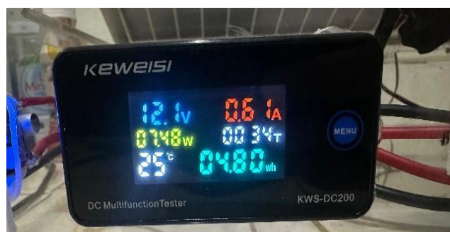
Gambar 2. 5 Digital Power Meter
