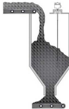
Gambar 2.6. Desain Coal bunker PLTU
