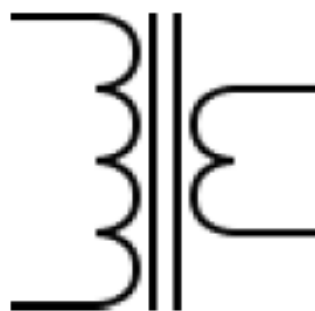
Gambar 2. 23 Skema Transformator Step-Down
