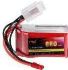
Gambar 4.7 Baterai Lipo 850mAh 3S 11.1V
