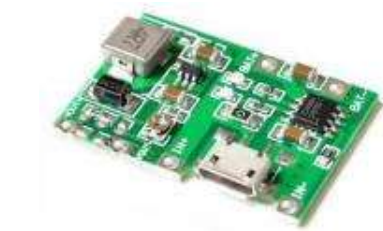
Gambar 4.5 Modul charger TP4056
