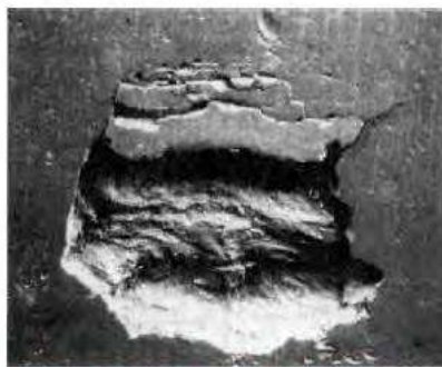
Fatigue failure of a steel ball bearing
