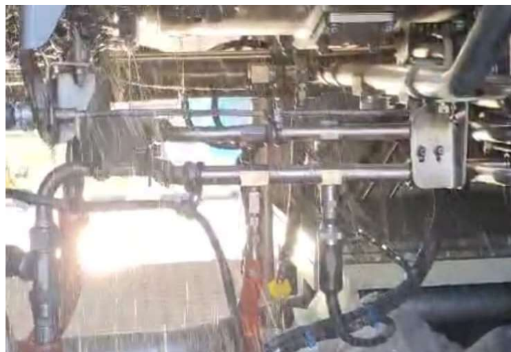
Gambar 2.19 Proses Water Wash Compressor
