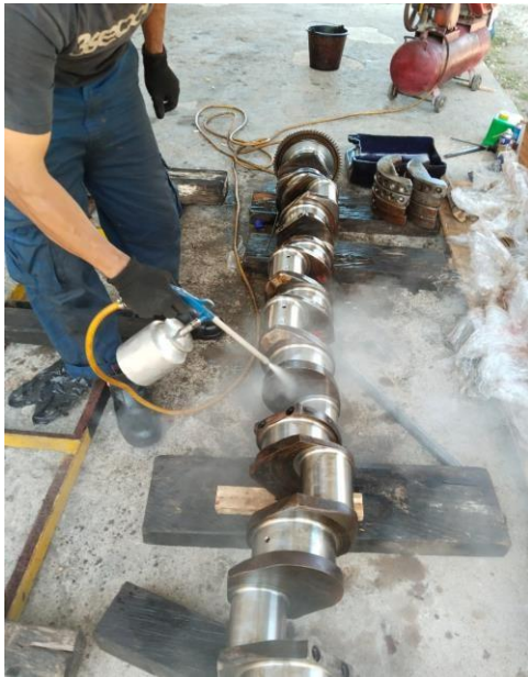
Gambar 2. 1.2 Poros Engkol Mesin SWD
