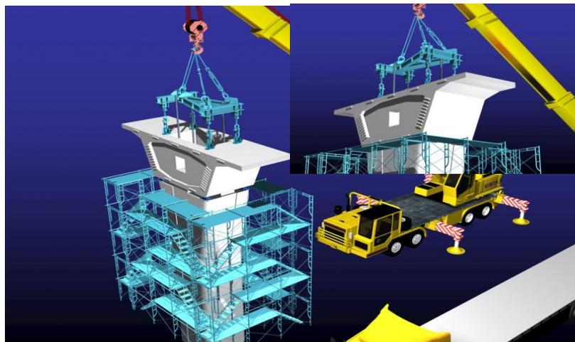
**Gambar 2.30** Peletakan *Box Girder Pier Segment*
