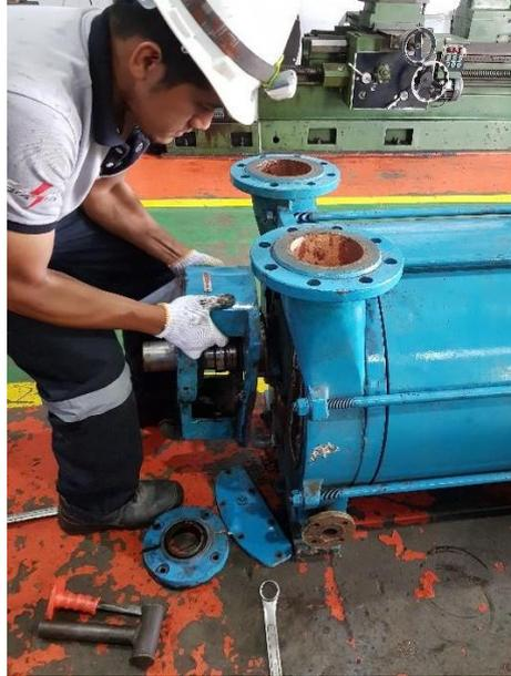
Gambar 4.4 Melepas first stage bearing cover
