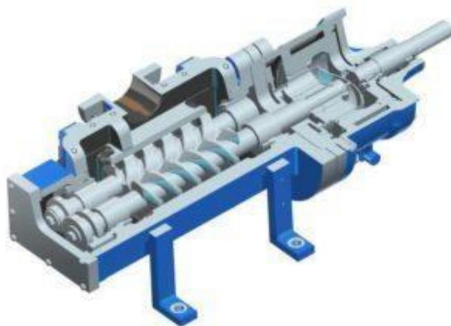
Gambar 2.13 Pompa Screw
