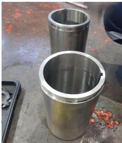
Gambar 4.12 Shaft Sleeve Baru
