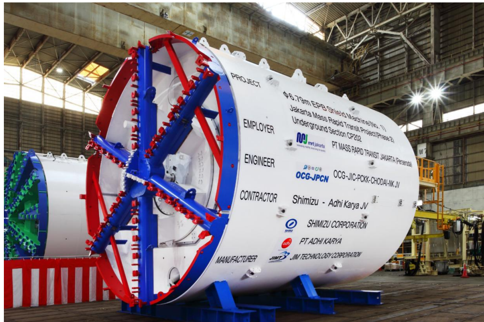
Gambar 2.1 Mesin Earth Pressure Balance (EPB)
