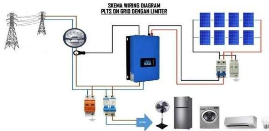
Gambar 2. 4 Sistem Plts On Grid
