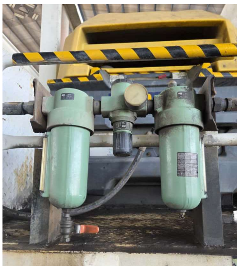
Gambar 2.7 Air Filter Double Regulator
