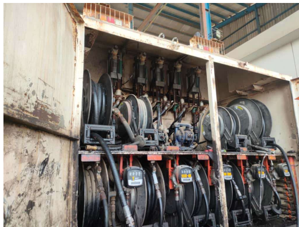
Gambar 2.4 Box Attachment Bagian Belakang Unit Lube Truck
