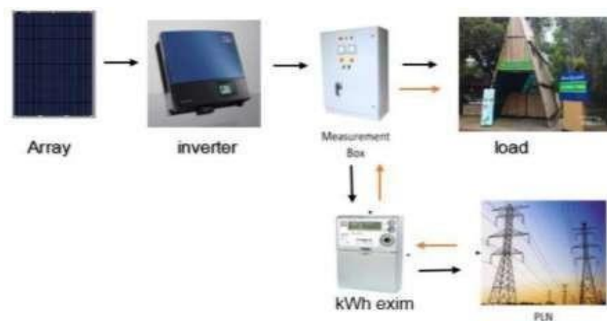
Gambar 2. 1 Blok diagram PLTS On Grid (Hutajulu et al., 2020)
