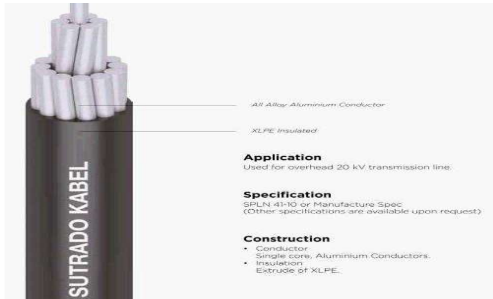
Gambar 2. 9 All Aluminium Alloy Conductor
