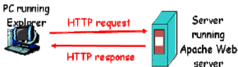
Gambar 2.7 Mekanisme Request – Reponse Web HTTP
