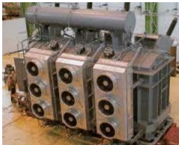
Gambar 2.5 Sistem pendingin Transformator.
